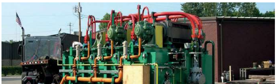
8-RF-pump drive for the 10,000-tonne closed-die forging press at Standard Steel (USA)
