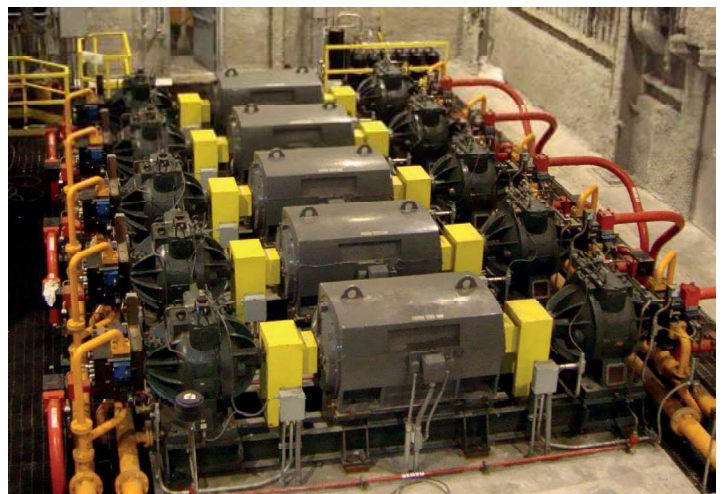
10-RX-pump PMSD drive for a 53 MN open-die forging press at Union Electric (USA).
